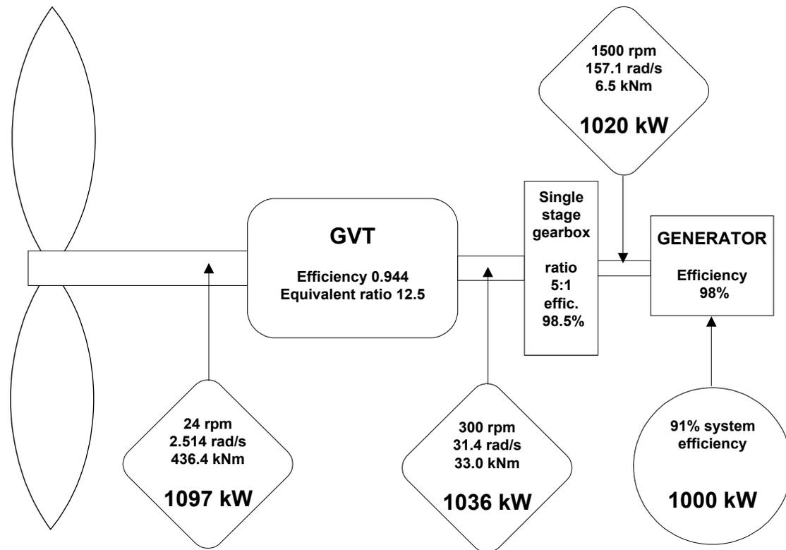
**Figure 2.2.2 Equivalent system with GVT and single stage gearbox**
