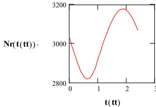
**Figure 4.4.1 Gyro speed [rpm] with no applied torque**
