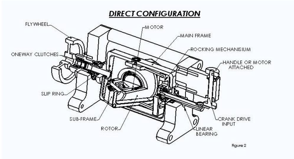
**Figure 5.1.1 Model of direct configuration**
