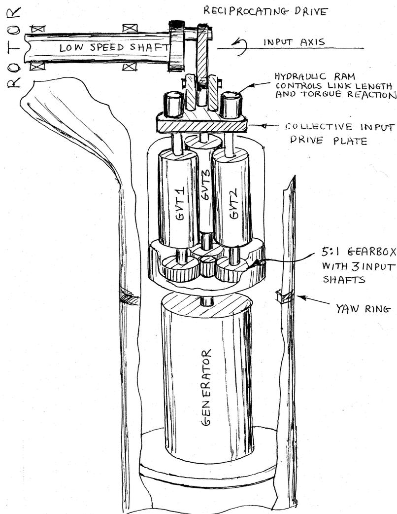
Figure 6.6.1 Preliminary layout of a GVT transmission for a wind turbine
