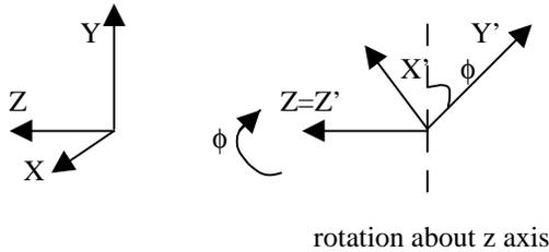
$x'$ ,  $y'$  and  $z'$  axes are fixed with respect to mainframe as shown below,
