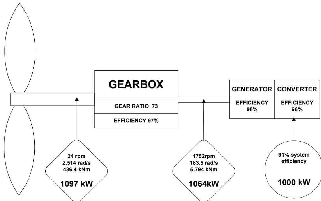
**Figure 2.2.1 Typical 1MW wind turbine variable speed transmission system**
