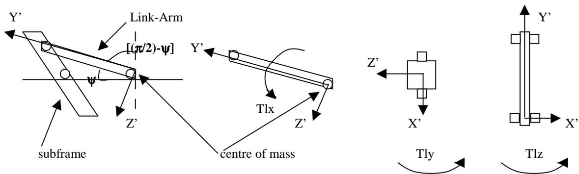
$T_{lx}$ ,  $T_{ly}$  and  $T_{lz}$  are torques acting on link-arm due to bearings.
