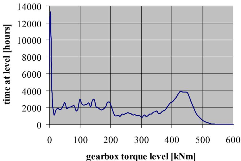
**Figure 3.2 Gearbox torque – time at level distribution**
