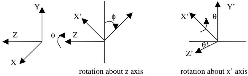
x' y' z' axes fixed with respect to subframe, as shown below. When  $\phi=\theta=0$ , x, y, z axes and x', y', z' axes coincide.
