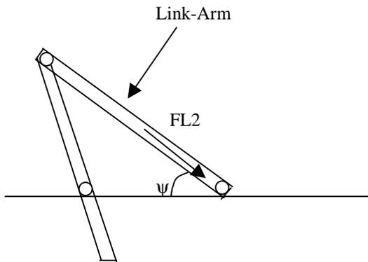
Differential forces at the bottom bearing of the link-arm.
